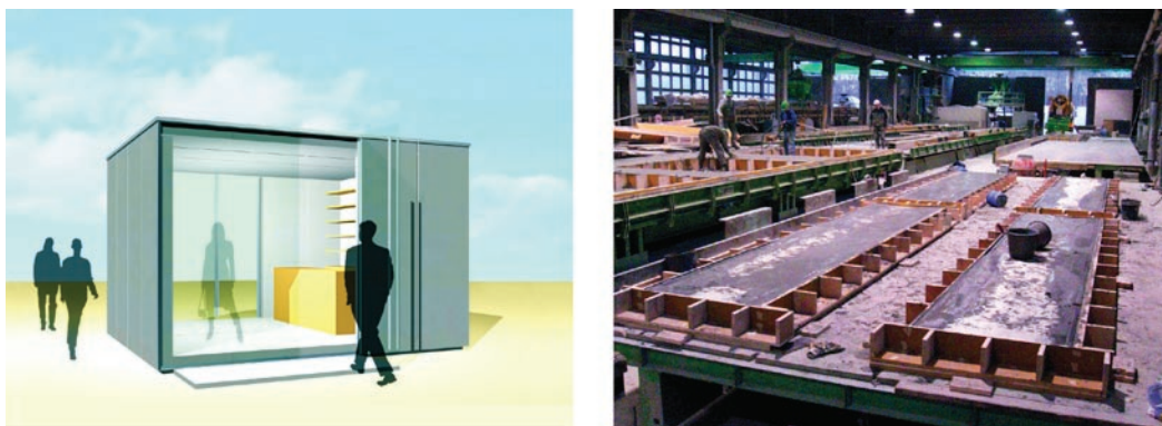
Figure 9: Architectural design of modular sandwich building and production of roof elements in precast company
