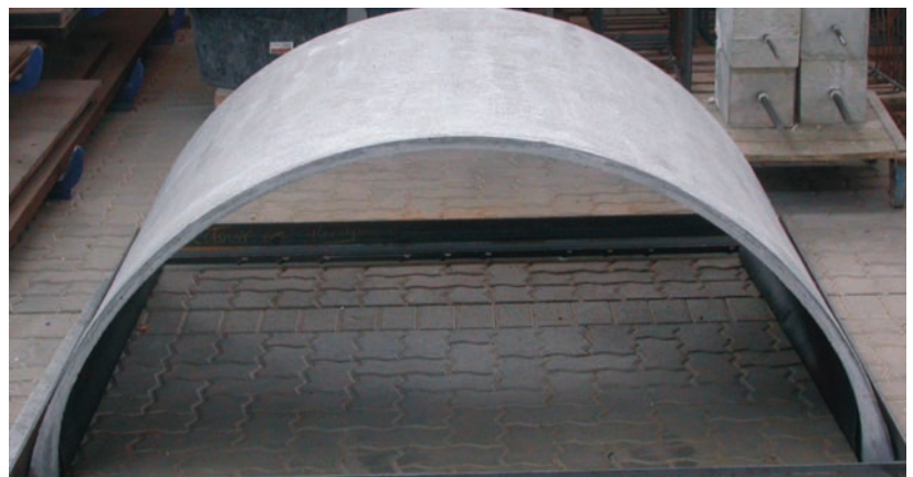
Figure 16: Prototype of the barrel shell made of TRC (ibac)
