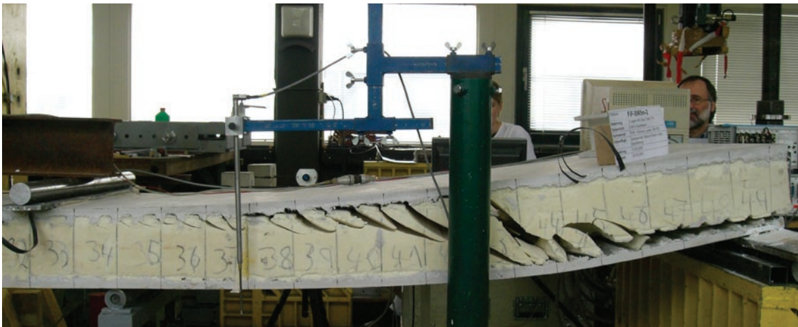
Figure 8: Shear failure of panel P4
